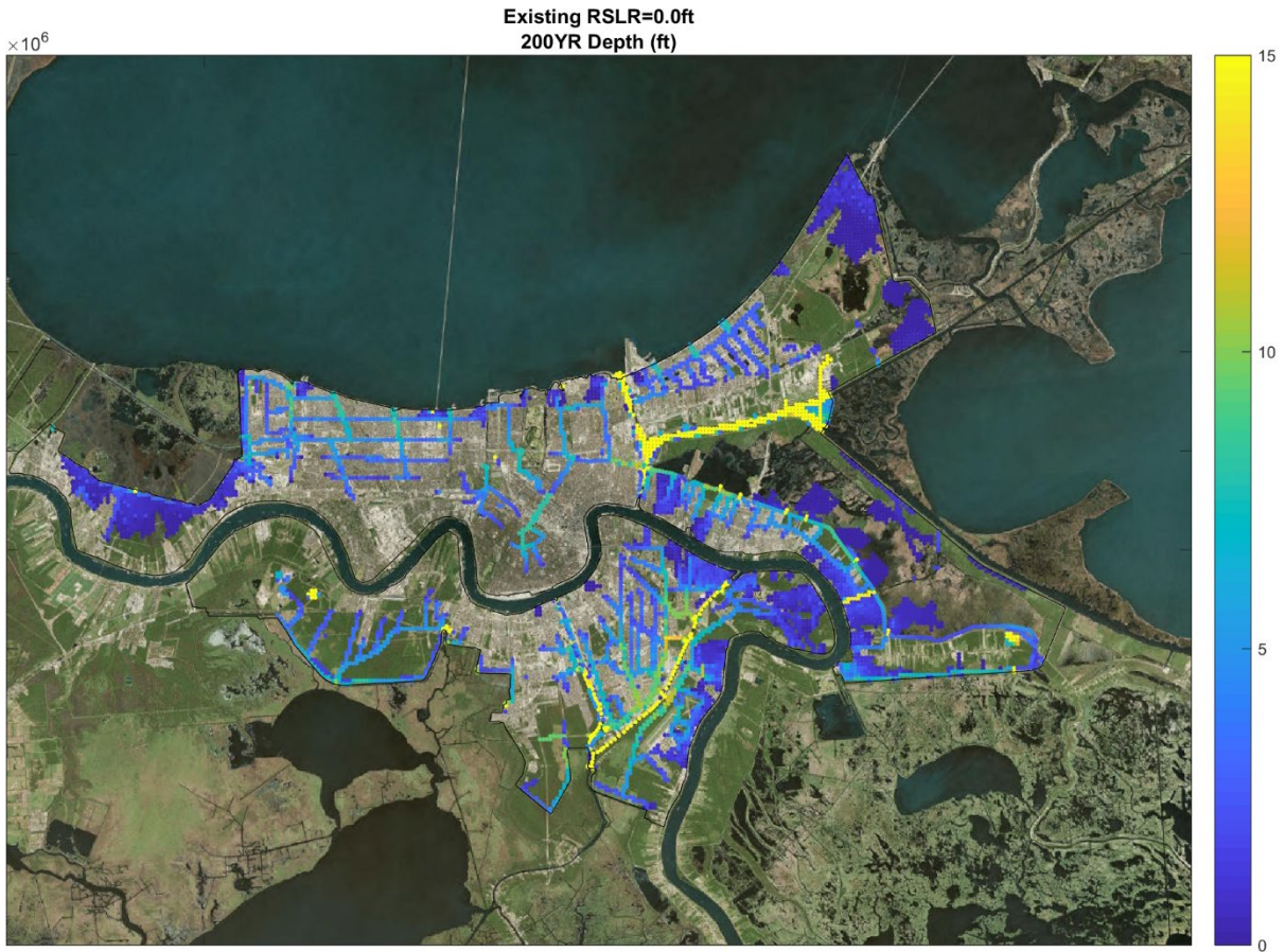
Figure 3-3. 0.5% AEP Peak Depths (ft.) for Existing Conditions
