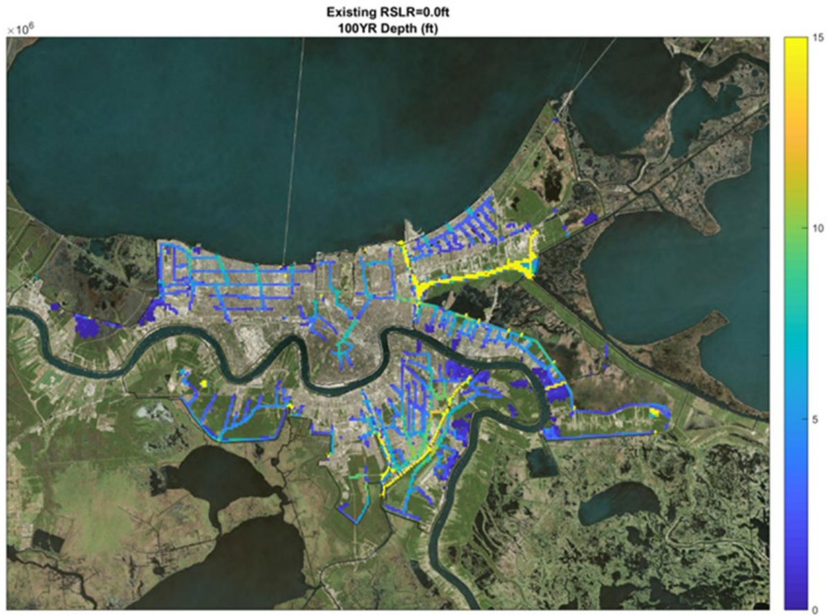
Figure 3-2. 1% AEP Peak Depths (ft.) for Existing Conditions
